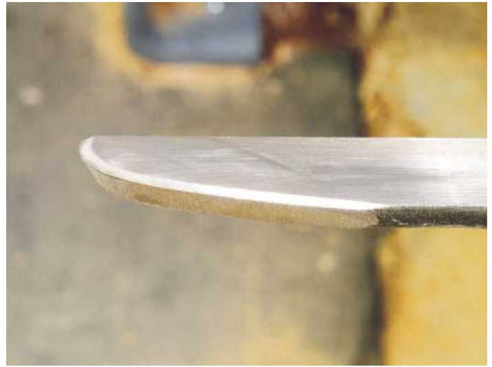
▲ Pic.2 Sharpening the tool is best done by completing the top surface first. Set your platform up so you take about 4mm off the top edge. The cutting bevel on the other side is ground in the normal way
